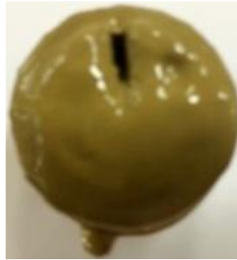
Figure 10. Top view of the fractured sandstone core plug at the end of the experiment no. 1.
