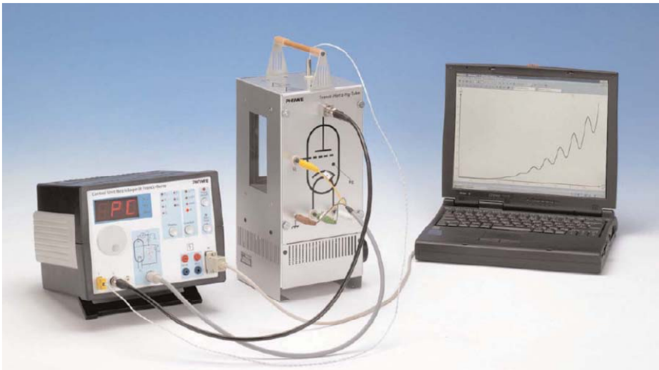
Fig.1: Set-up for the Franck-Hertz experiment with PC.
