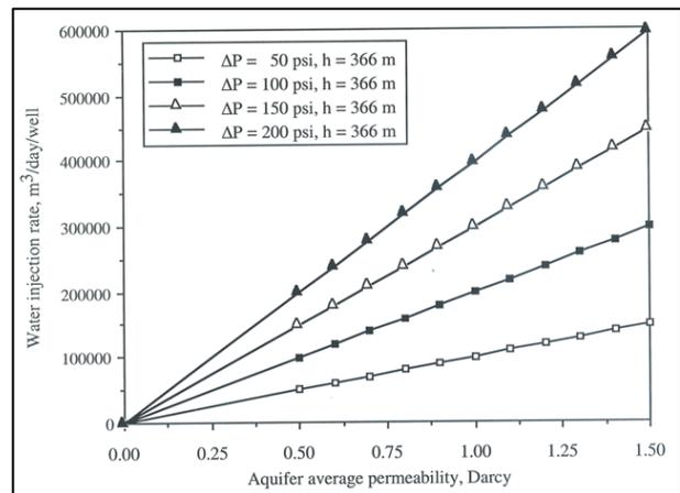
Fig. 4. Relationship between aquifer average permeability, pressure drop and water injection rate.
