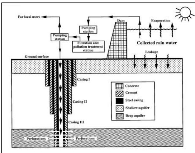
Fig. 3. Schematic diagram of a suggested groundwater artificial recharge station.
