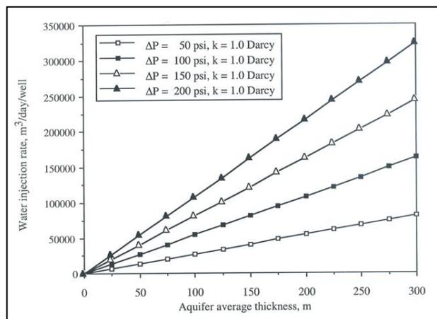
Fig. 4. Relationship between aquifer average thickness, pressure drop and water injection rate.
