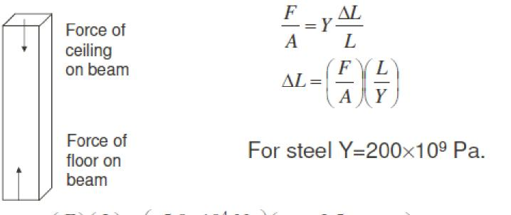
$$\Delta L = \left(\frac{F}{A}\right) \left(\frac{L}{Y}\right) = \left(\frac{5.8 \times 10^4 \text{ N}}{7.5 \times 10^{-3} \text{ m}^2}\right) \left(\frac{2.5 \text{ m}}{200 \times 10^9 \text{ N/m}^2}\right) = 1.0 \times 10^{-4} \text{ m}$$
