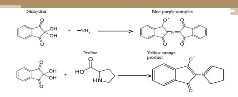
It destroys each primary  $\alpha$ -amino acid and also reacts with the released NH3 to form a deep purple chromogen referred to as **Ruhemann's Purple**, which has a maximum absorption at about 570 nm.
