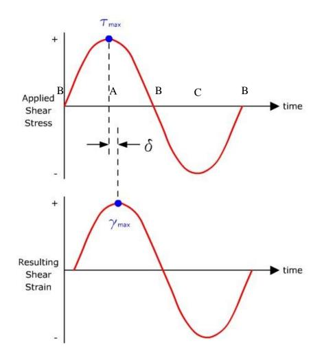
In this procedure, a disk of asphalt cement is placed between an oscillating spindle and the base plate. Since asphalt cement is a viscoelastic material, there is a time lag ( $\delta$ ) between the applied shear stress and the resulting shear strain. This is shown in Figure above. The maximum shear stress ( $\tau_{max}$ ) and the maximum shear strain ( $\gamma_{max}$ ) are calculated using the following equations:
