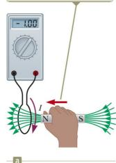
When the magnet is held stationary, there is no induced current in the loop, even when the magnet is inside the loop.
