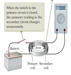
❖ The emf induced in a circuit is directly proportional to the time rate of change of the magnetic flux through the circuit.
