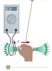
Experimentalists, Faraday and Henry et al., found that an emf is induced in the circuit if the magnetic flux through the surface bounded by the circuit is changed.
