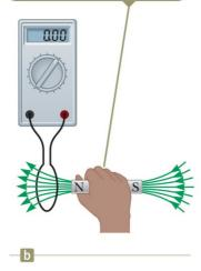
When the magnet is moved away from the loop, the ammeter shows that the induced current is opposite that shown in part a.
