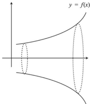
But rather than take a cross-section, let us take a thin disc of thickness  $\delta x$ , with the face of the disc nearest the y-axis at a distance  $x$  from the origin.
