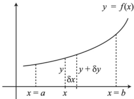
The radius of this circular face will then be  $y$ . The radius of the other circular face will be  $y + \delta y$ , where  $\delta y$  is the change in  $y$  caused by the small positive increase in  $x$ ,  $\delta x$ .
