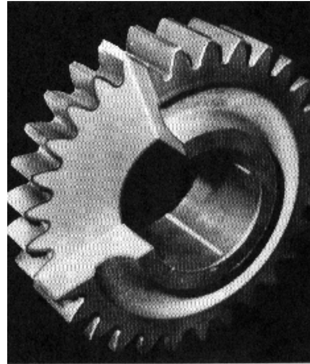
a case hardened gear
