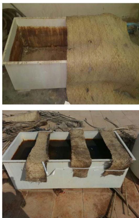
Fig. 1. Sample Photos of the Used Rectangular Tanks and the Coverage Patterns: (a) ½-covered, (b) Strips-covered
