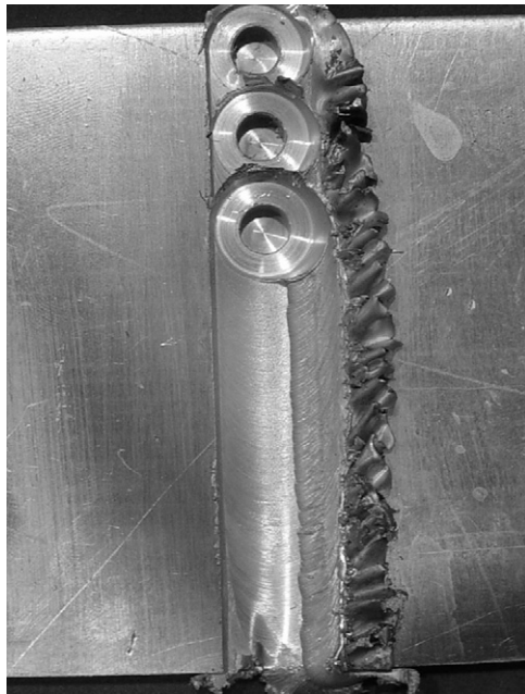
Fig. 1. FSP'ed sample using 3–100% overlapping passes.
