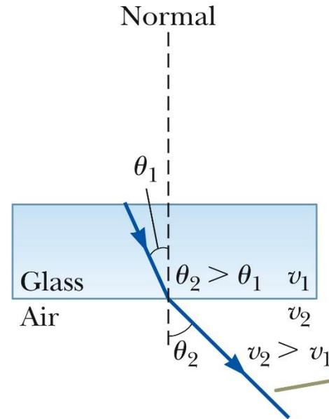
When the beam moves from glass into air, the light speeds up upon entering the air and its path is bent away from the normal.
