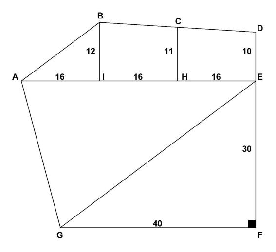
Assuming coordinates of point A: (x=0.0m, y=0.0m) with AE as the x-axis, use method of coordinates to compute the total area.
