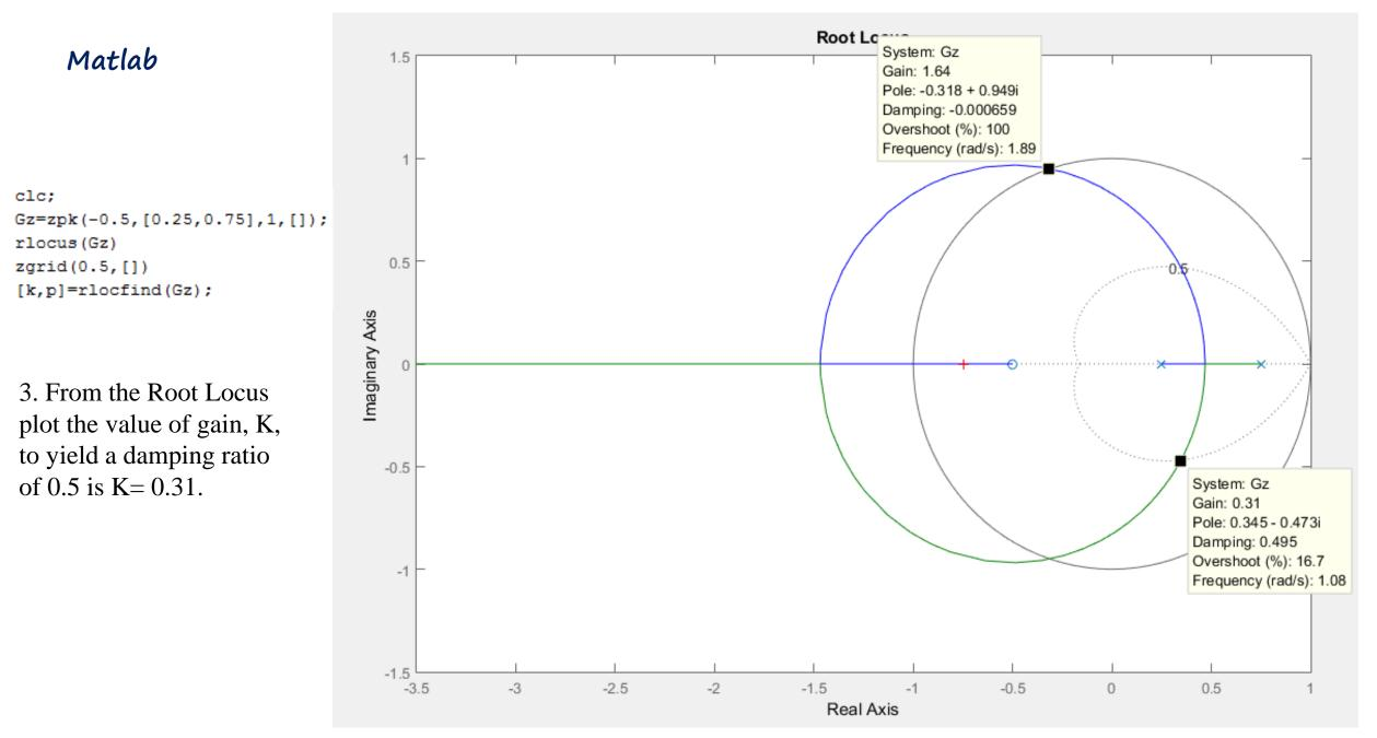
A lead compensator  $G_c(s)$  is designed for a unity feedback system whose plant is
