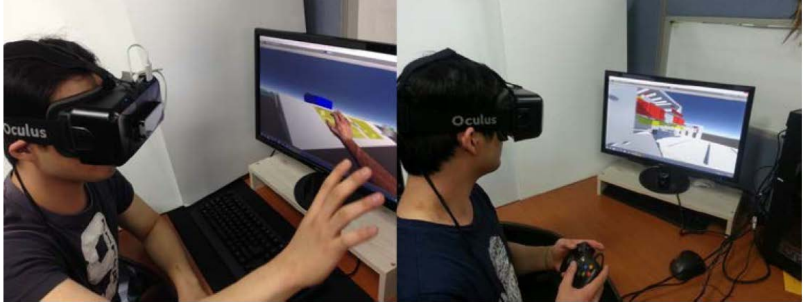
Figure 7. Controlling the 3D virtual environment with Oculus Rift and Leap Motion (left) and controlling the 3D virtual environment with Oculus Rift and Xbox controller (right) during the Iteration 1
