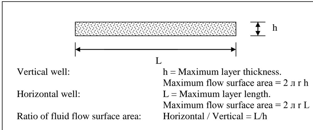
**Figure 1. Available flow surface areas for vertical and horizontal wells drilled in the same formation.**
